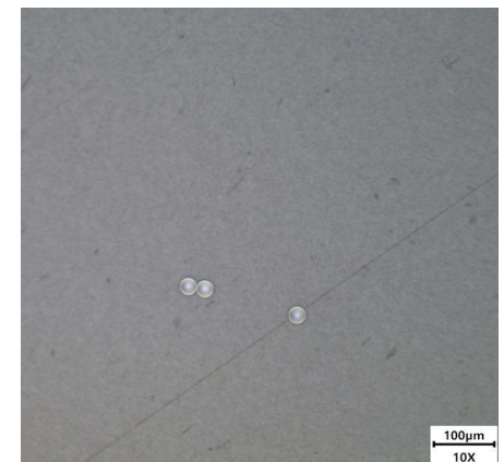
Figure 5: Microscopic image showing NIST traceable polystyrene microsphere control sample prepared by laboratory for QC purposes.
