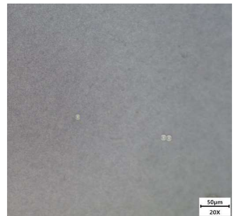
Figure 4: Microscopic image showing NIST traceable polystyrene microsphere control sample prepared by laboratory for QC purposes.
