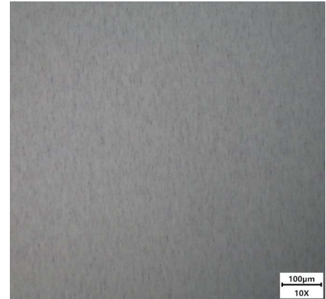
Figure 3: Microscopic image of 100ml filtered laboratory prepared particle free water used for sample preparation, filter rinse and glassware cleaning. No microplastic particles are detected.
