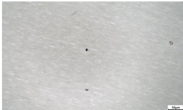
Figure 2: Microscopic images showing mineral grains and organic dust in sample 107-21986 with no evidence of microplastics.
