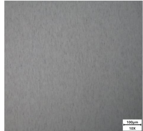
Figure 3: Microscopic image of 1000ml filtered laboratory prepared particle free water used for sample preparation, filter rinse and glassware cleaning. No microplastic particles are detected.
